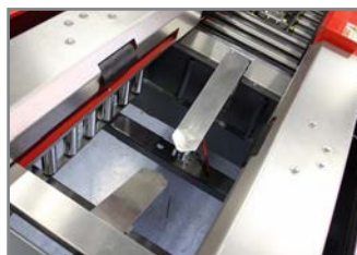
SISTEMA CHIUDI FALDE FLAP CLOSING SYSTEM
