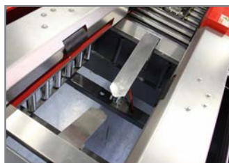
SISTEMA CHIUDI FALDE FLAP CLOSING SYSTEM
